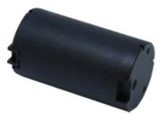
The LVC (Linear Vibration Components) series achieves wideband and clear vibrations by suppressing higherorder resonances through its unique spring and damping structures. It also applies the principle of voice coil (VCM) and can produce sound by directly vibrating surfaces such as panels. This allows for the addition of speaker functionality while minimizing the impact on the design by mounting it on the back of the housing.
