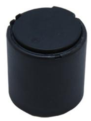
The LVC (Linear Vibration Components) series achieves wideband and clear vibrations by suppressing higherorder resonances through its unique spring and damping structures. It also applies the principle of voice coil (VCM) and can produce sound by directly vibrating surfaces such as panels. This allows for the addition of speaker functionality while minimizing the impact on the design by mounting it on the back of the housing.
