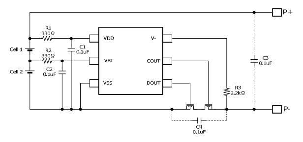
R1, C1, R2, C2 stabilize a supply voltage ripple. However, R1 is enlarged, the detection voltage shifts by voltage when c urrent consumption flows into R1. Please decide it after confirming the characteristic. Moreover, adjust the value of C1, C2 to 0.01uF or more to do the stability operation, please.
