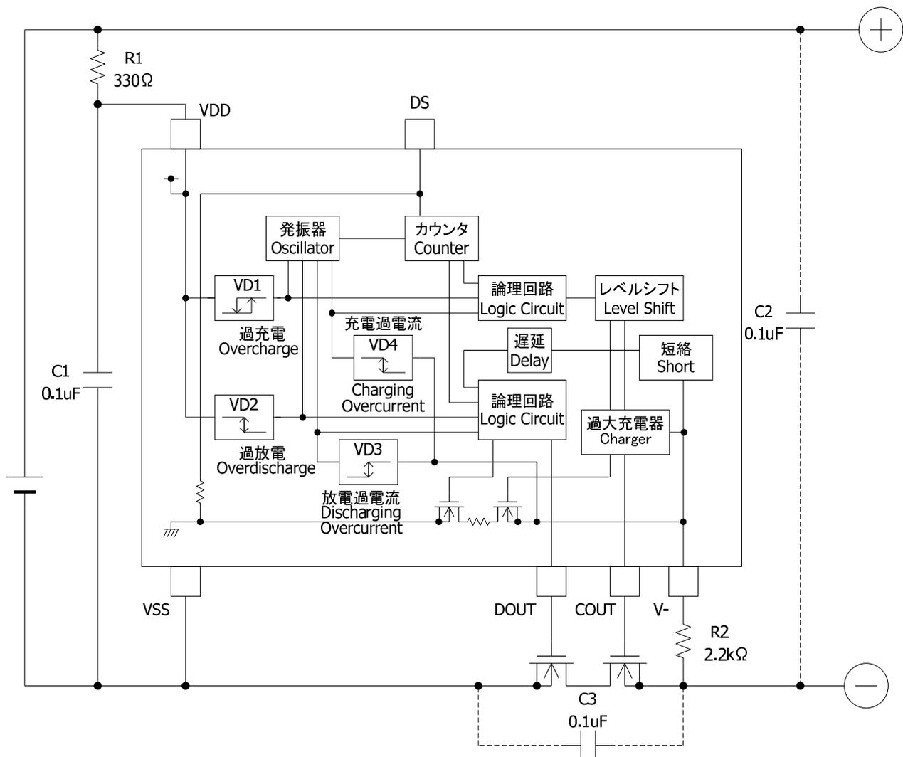
R1 and C1 stabilize a supply voltage ripple. However, the detection voltage rises by the current of penetration in IC of the voltage detection when R1 is enlarged, and the value of R1 is adjusted to 1kohm or less. Moreover, adjust the value of C1 to 0.01u
