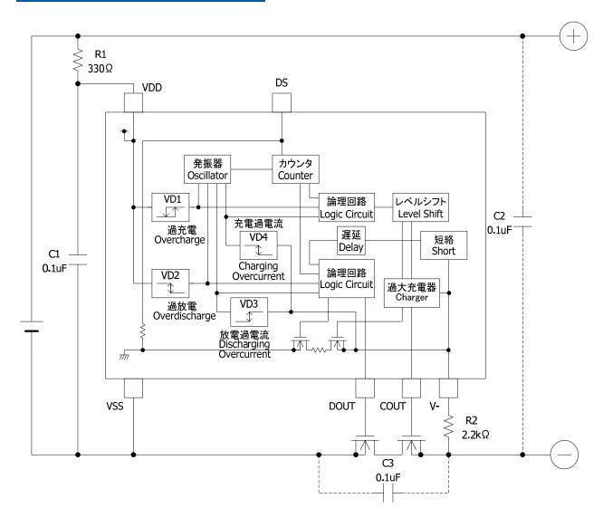
R1 and C1 stabilize a supply voltage ripple. However, the detection voltage rises by the current of penetration in IC of the voltage detection when R1 is enlarged, and the value of R1 is adjusted to 1kohm or less. Moreover, adjust the value of C1 to 0.01u
