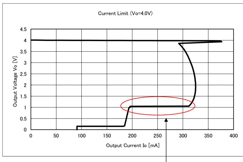
The current limit operate in this area (half short  $1.8\sim 3.6\Omega$ ).
