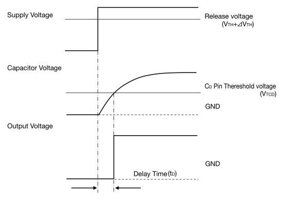
Delay Time(t<sub>D</sub>) PST89XA Series (10MΩ) RD: CD Pin Resistance  $t_D \doteq 0.69 \times RD \times CD(F)$  (s) CD: Capacitor
