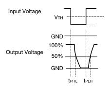
$V_{TH}=1.2V$ ,  $1.3V \rightarrow Input Voltage V_{TH}=0.3V \sim V_{TH}+0.3V$ VTH=1.4V~5.2V → Input Voltage VTH-0.4V ~ VTH+0.4V
