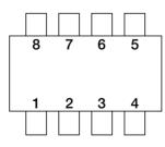
SOP-8C/DIP-8B (TOP VIEW)
