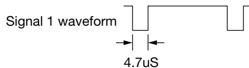
\*2 Measuring horizontal sync signal pull-in range for NTSC
