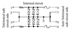
1,4,5,8: Terminals for signal wiring 2,3,6,7: Terminal for grounding
