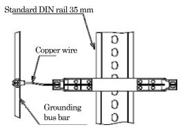
Mounting to installation panel (Apply the optional socket.)
