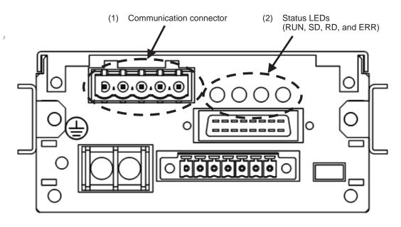
$(1) \ Connector \ board \ of \ the \ communication \ connector$
