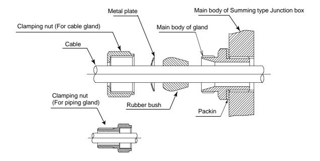
Note) In case of application of SB-310-B type, only the clamping nut will become as the above figure indicates.
