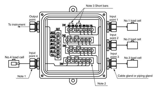
Note 1) In case of 3 points of application, input point 4 is seal plug.
