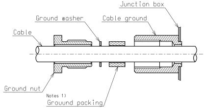
Notes 1) According to the diameter of a cable, as shown in the following table, please use the ground packing property.
