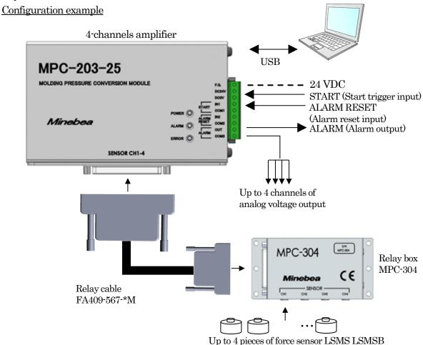
\*This unit can be also used by connecting the relay box MRB-304-BI or MRB-304-CV.
