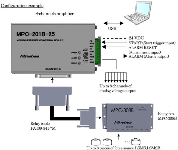
\*This unit can be also used by connecting the relay box MPC-308,MRB-304-BI and MRB-304-CV.
