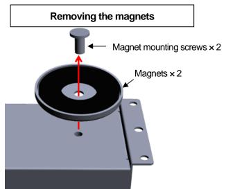
Remove the magnets before mounting using the bolts. The magnets can be removed by removing the screws in the center of the magnets.
