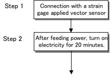
Connect the instrument with a strain gage applied vector sensor.
