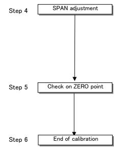
Load standard weights (use them as near as the standard weights) on whichever one axis in Fx axis, Fy axis and Fz axis, then adjust with the GAIN trimmer for the corresponding axis so that the voltage output value to be set shall be obtained.
