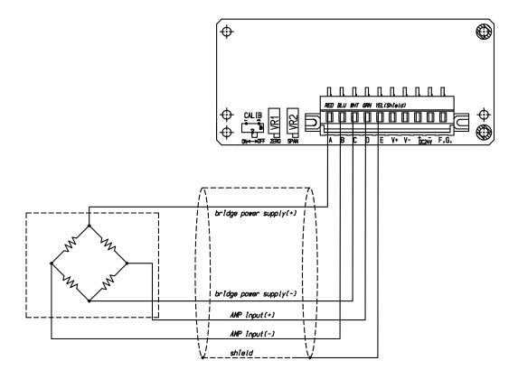
This instrument is avairable to connect with extension type junction box B-304B. Connect of one gage type transducer, junction box B-304, and CSA-528.
