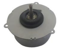
dia. 92.5(max dia. 105) × L44.5 DC Brushless motor outer rotor type (B) dia. 92 × L45 DC Brushless motor outer rotor type Motor Type : 3 Phase DC Brushless Motor Direction of Rotation : CW and CCW Control-Driver circuit built-in. Compact, Light Weight and High Output High Efficiency Low Noise Overcurrent and Locked Rotor Protection
