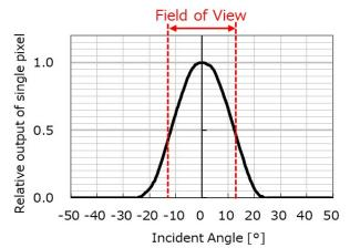
Field of View (FOV): defined as the angular range of inceident infrared ray at half signal point.
