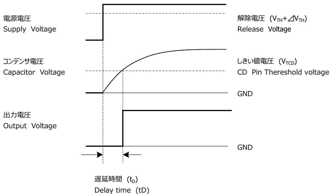
遅延時間( $t_D$ )  $t_D = 0.69 \times R_D \times C_D$  (s)
